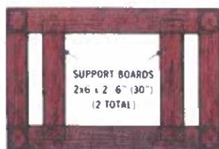
UNDERSIDE VIEW (Showing Support Boards)
